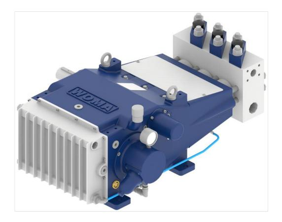
The high-pressure plunger pumps of the 2-series with operating pressures up to 750 bar and flow rates up to approx. 224 l/min, are ideal for the cleaning of pipes and tube bundles, vessels and containers. Variant V of the 2-series has been specially developed for applications with elevated inlet pressure.
