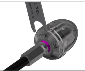
The rotating speed can be adjusted, depending on the level of deposit. DERC SPC is available in three sizes: SPC-L, SPC-M and SPC-S. The SPC-L is designed and constructed for waterblast cleaning of pipes as small as 6" with elbows and up. The SPC-M is for cleaning 4" pipes. And the SPC-S is made for the same work in pipes as small as 2" with elbows.
